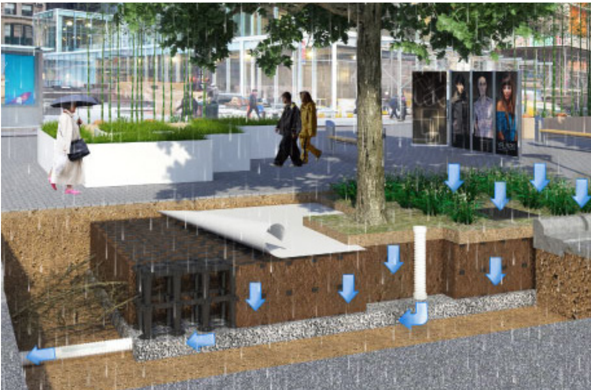
Figure 2. Strataflow™ Raingarden Stormwater Treatment/Storage System
