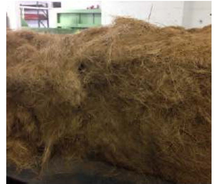
Brown Coir Lightly Misted for Log Production Coir Logs contain the brown coir compacted in to a tubular or rectangular net as shown above
