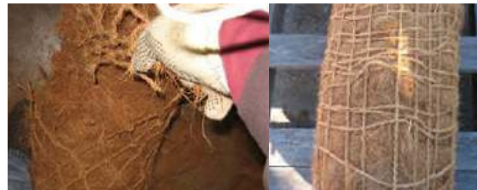
Attempt to Compact 12" Natural Coir Net to 9 lbs/ft 3 Density Inconsistent Netting
