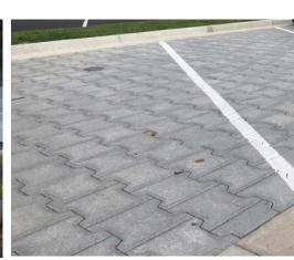
PowerBLOCK is an open-joint permeable paver system that moves rainfall through pavement up to 10 times faster than traditional permeable/porous systems. With a guaranteed surface infiltration rate of over 1,000 inches per hour, PowerBLOCK provides a drivable surface that requires minimal attention from project owners.
