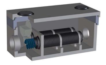
Each Helix filter column has a designed treatment flow rate of approximately 3 cubic feet/sec. Helix filters are offered as single, double and triple column systems. Filter cartridges are replaceable and can be accessed through a standard 36" diamater manhole provided in the vault.
