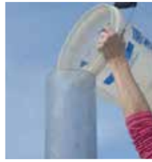
Figure 9: Filling Infiltrator with Water
