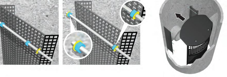
With Trash Guard Plus in place, attach side mesh panels to side of Trash Guard Plus with 4 tie wraps and 6 washers and 6 nuts as shown.
