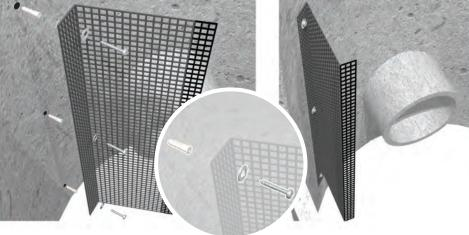
Position Trash Guard Plus in place and slide steel rods through holes in Trash Guard Plus<sup>®</sup> to mark assembly position on wall with chalk as shown.
