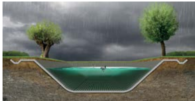
Stormwater holding and storage basins
