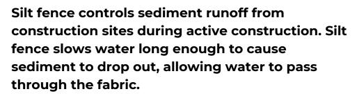
Silt fence is made of a woven polypropylene material and is nonbiodegradable. This engineered geotextile is stabilized to resist degradation due to ultraviolet exposure. It is resistant to commonly encountered soil chemicals, mildew, and insects. Polypropylene is stable within a pH range of 2 to 13, making it one of the most stable polymers available for geotextiles today.
