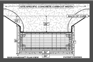
SLAB DIMENSIONS, DISTANCE FROM CURB, AND CHAMBER ELEVATION VARIES WITH SITE CONDITIONS. THE TOP OF THE METAL GRATE, HOWEVER, SHOULD BE 1.5" - 2" BELOW THE GUTTER AND THE CONCRETE SLAB SHOULD EXTEND WELL BEYOND THE FILTER WALL TO SERVE AS A SPLASH DISSIPATER.
