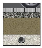
Provide water quality treatment by incorporating a sand layer or innovative media below the surface.
