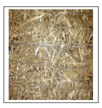
WintersChoice™ Products are extended-term, double net erosion control blankets that are machine-assembled using a blend of 70% agricultural straw and 30% coconut fibers. These fibers are evenly distributed throughout the entire area of the blanket to a rough thickness of 1/2″ and stitched between biodegradable jute netting using biodegradable cotton thread. Biodegradable thread is used on all of our Bio (Jute) products.
