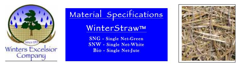
WinterStraw<sup>™</sup> Single Net Products are short term, single top net erosion control blankets that are machineassembled using 100% agricultural straw fibers. The straw fibers are evenly distributed throughout the entire area of the blanket to a rough thickness of 3/8″ and stitched to your choice of netting using high strength degradable thread. Biodegradable thread is used on our Bio (Jute) products.
