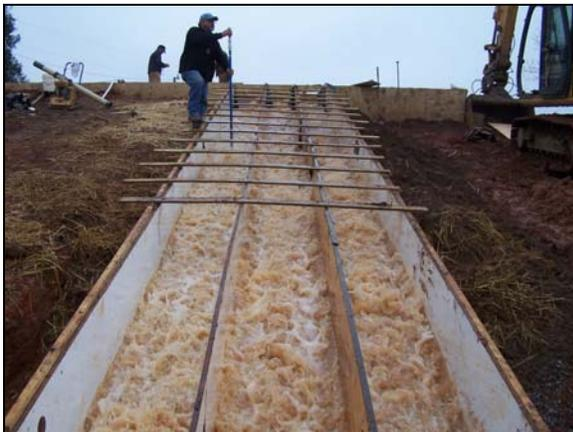
Figure 3. Channel Flow Velocity Measurement (typical)
