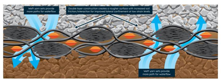
Unique double layer construction of MIRAFI RSi-Series consisting of monofilament and fibrillated yarns to provide more than three times the surface area of a typical woven geotextile
